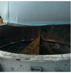
The bag is opened by cutting a cross in the bottom of the bag by using either a knife or an emptying device in which a knife and a screen are mounted.
