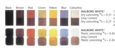
The shades of coloured Dry concreting W/c = 0.27 concrete depend not only on the cement used in the Dry concreting W/c = 0.27 concrete. The w/c ratio has a major influence.
